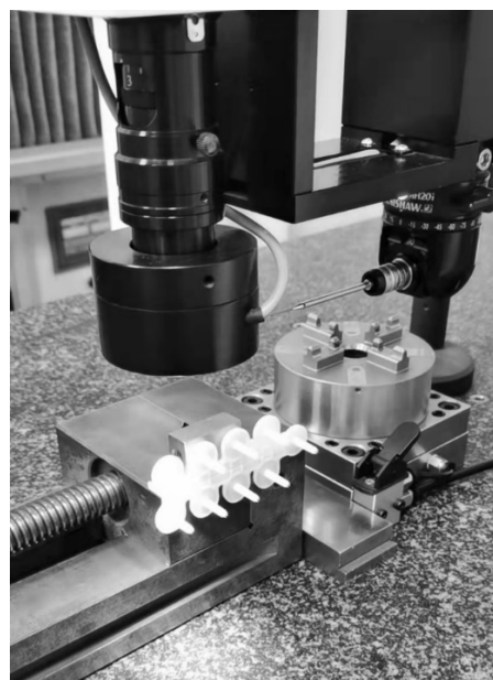
Figure 1. Coordinate Measuring Machine set up in preparation of tine length and diameter measurements.
